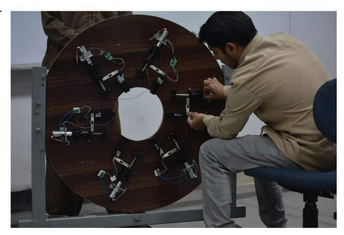
The indenter device employs 9 degree of freedom (DOF) system six for linear actuators one passive rotational degree of freedom and two for frame translation motion. It contains 6 position and force controllable linear actuators .These actuators surround the limb in circumferential ring.
