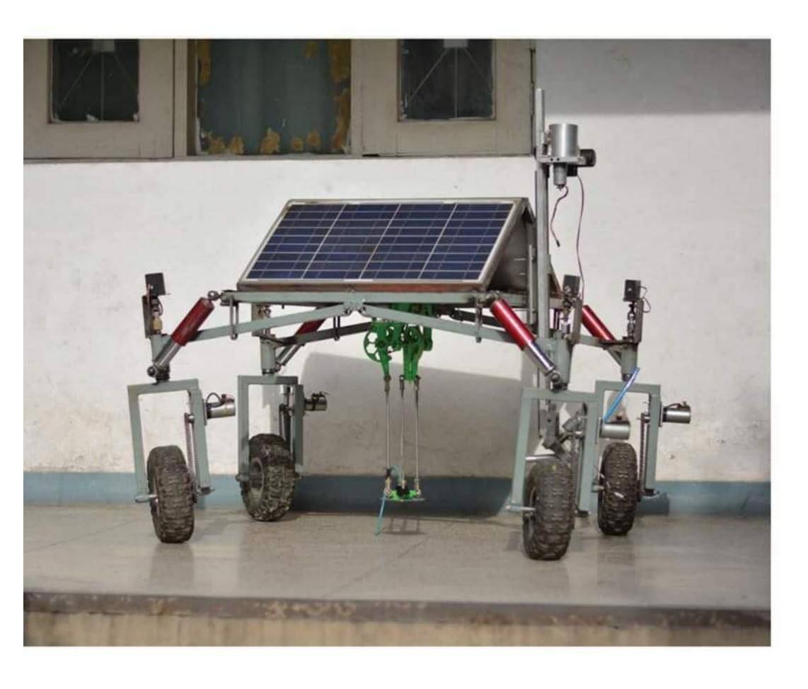
The end effector is designed to be a multipurpose, adjustable tool to perform farming tasks while mounted on mobility platform. Delta robot is attached at the center of platform which detects the weeds and sprays on it. The robot is inputted by user about seed variety, it moves autonomously furrows and adjust the seeding depth and distance between it with performing of sowing and weeding operations.
