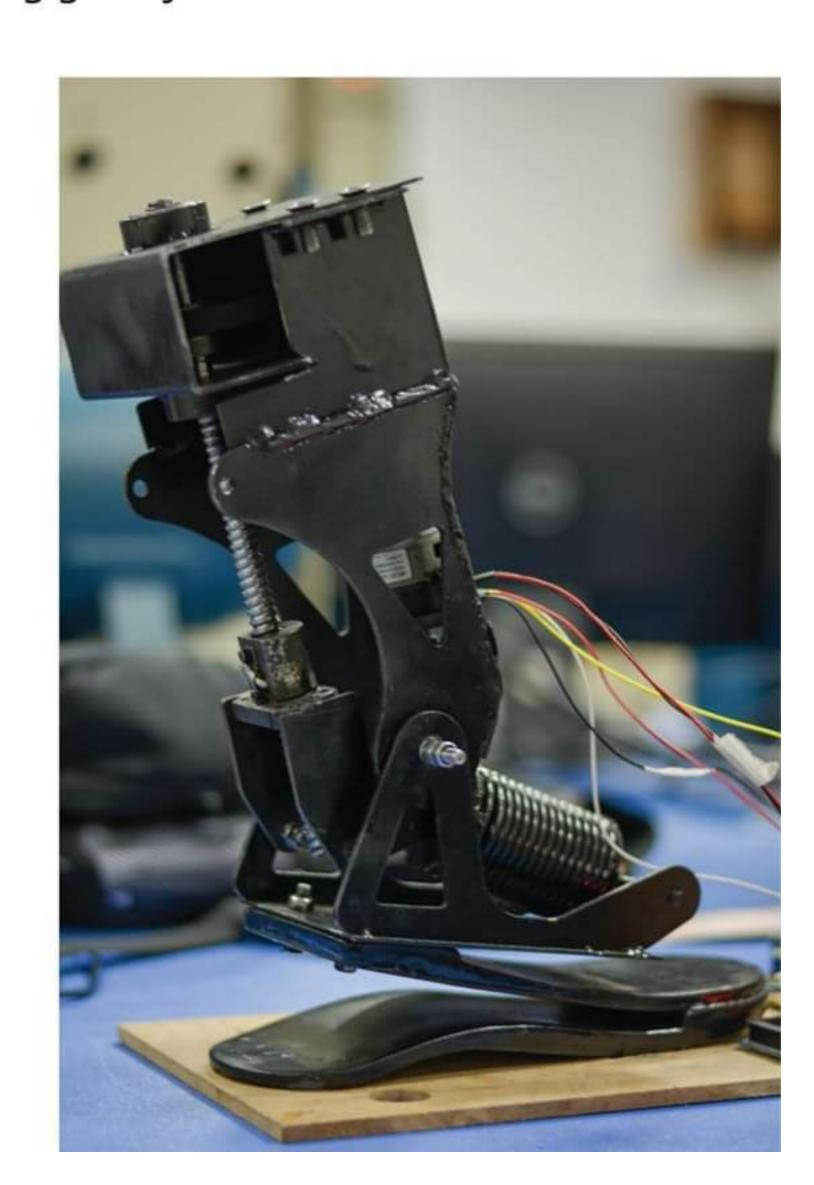
Despite of the conventional passive rigid link we are providing an active solution to implement Degree of Freedom in the ankle joint through mechanical components like Motor, Ball Screw, Pulleys and Belt Drive moreover also providing Variable Stiffness and Heel Cushioning by incorporating Shock Absorber and adding design constraints in basic structure.
