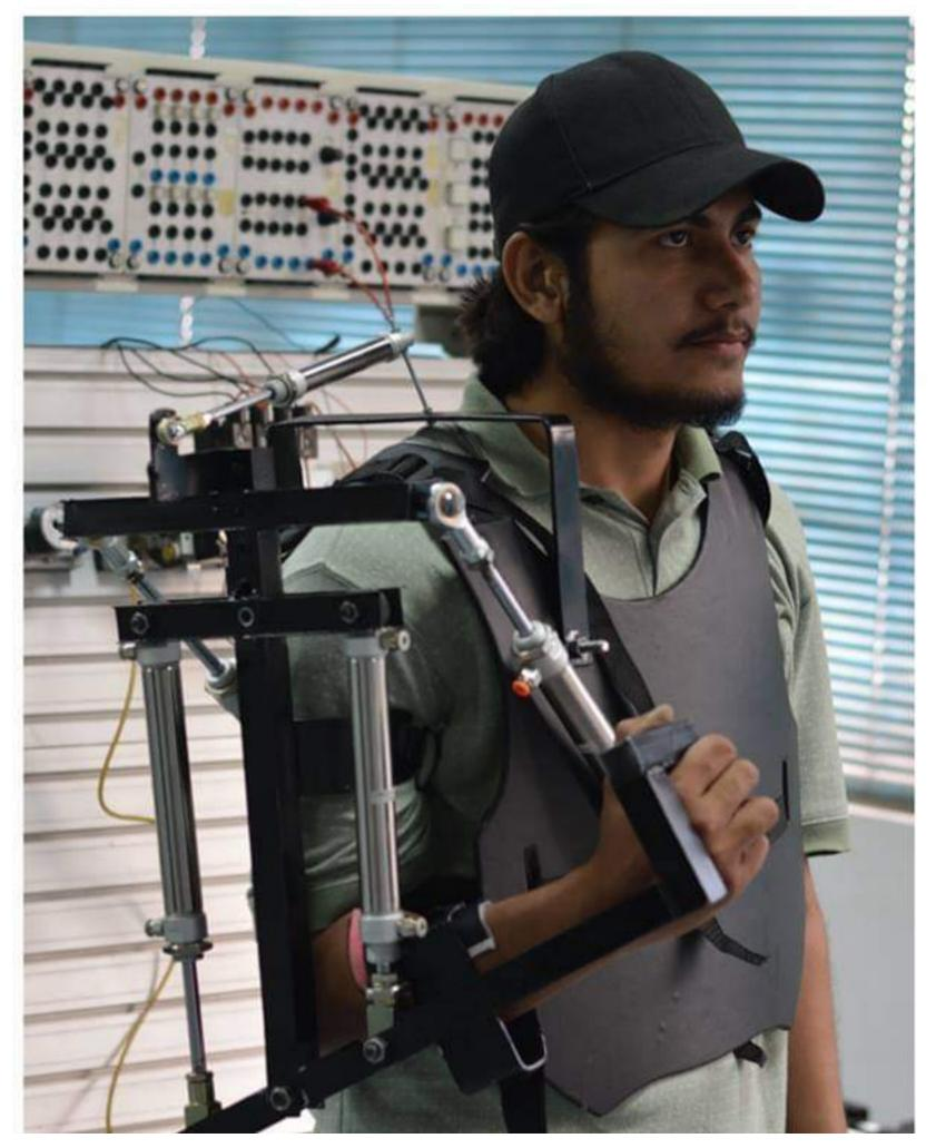
For this project, pneumatic cylinders along with 5/3 solenoid operated valves have been used. When a certain pressure is applied, the corresponding cylinder gives us the required motion through extension and retraction. The valves used are basically proportional valves that allow us to retain the position of cylinder at specific position. In the next step, 3D modeling is done using SolidWorks and then the stress analysis was performed.
