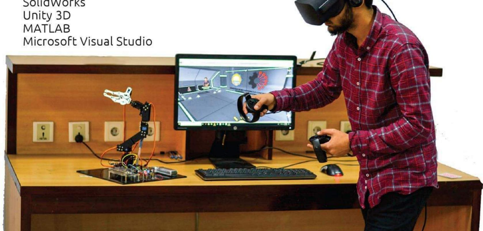
The virtual environment was created using Unity 3D software. The real robotic manipulator is also placed in the real world. A human operator uses the Oculus Rift headset which makes the operator feel like he is in a virtual world. The human operator may move the end-effector of the model of robotic manipulator in virtual environment using the Oculus controllers in any direction he wants.
